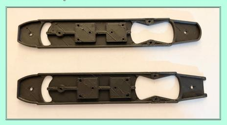
The next photo shows the 3D printed floor intended for the Bowser metal PCC shell compared to the metal floor, part #1283, made for that same shell. Looks like a winner so far!
